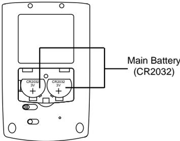
**WARNING:** Turn the unit off before replacing batteries. Replacing batteries when the unit is on may cause permanent damage. Replace the batteries within 1 minutes, or else, the time, city and language will be corrupted and you will need to input them again.
