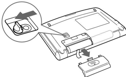
4. Remove the old batteries by pulling the ribbon tab.
